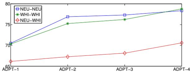
Figure 4: Accuracy of lipreading using adaptation. ADPT-1, ADPT-2, ADPT-3 and ADPT-4 give the results when the models are adapted with 1, 2, 3 and 4 samples per digit, respectively. The vertical axis gives the accuracy in percentage.
