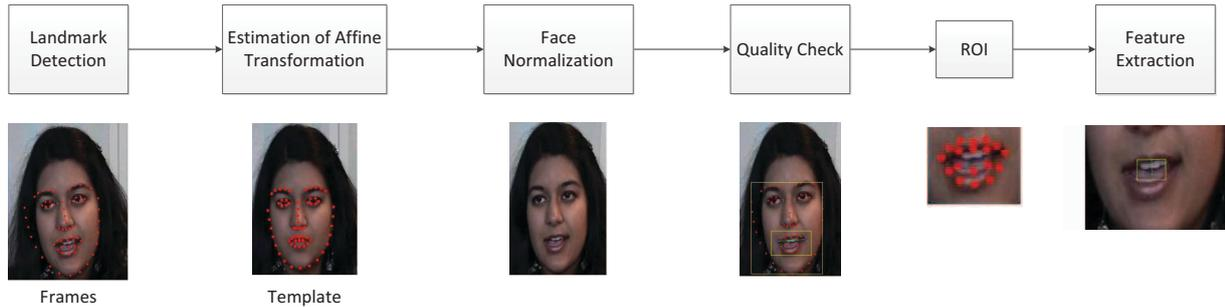
Figure 2: The block diagram to estimate facial features. Facial landmarks are detected using a deformable model that compares each frame with a template image. After normalizing head rotation, the location of the landmarks are evaluated during the quality control step. Finally, we determine the region of interest and we estimate the geometric and appearance based features.
