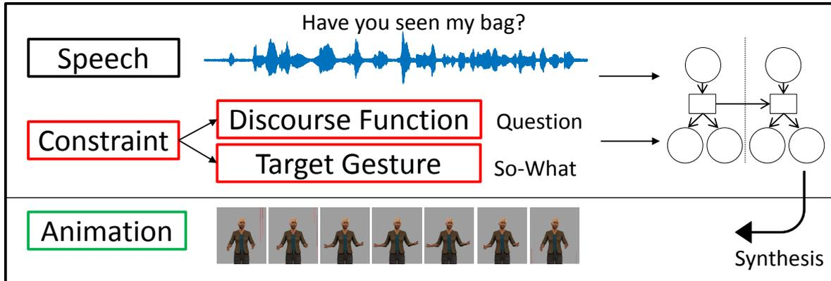
Figure 1. Overview of the proposed system to generate behaviors. In addition to speech, the models take constraints as input (either discourse functions or target gesture), generating meaningful data-driven behaviors.
