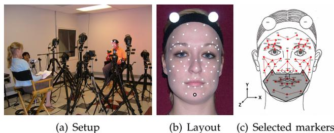
Fig. 3. (a) Recording setup for the IEMOCAP database, (b) layout of the motion capture markers in the IEMOCAP database, and (c) selected markers used in our previous analysis [2], which are used for emotion recognition experiments (Sec. 5).
