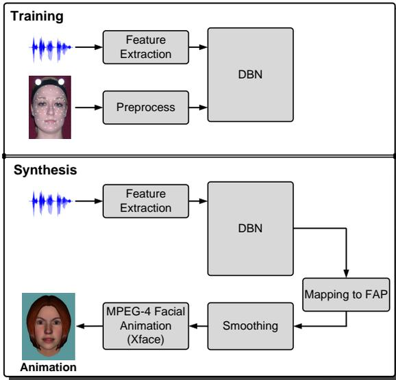
Fig. 5. Proposed system overview. Coupling between acoustic features and facial gestures are captured during training step. Inference process maps each sequence of acoustic feature to its visual counterpart. Finally, synchronized animation is generated with Xface.
