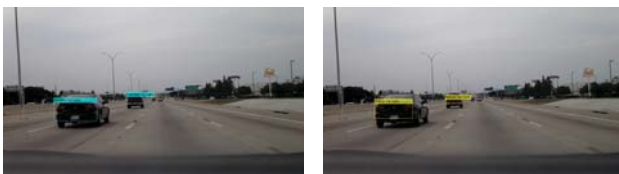
(a) Tail-light detector output (b) Manual annotation
