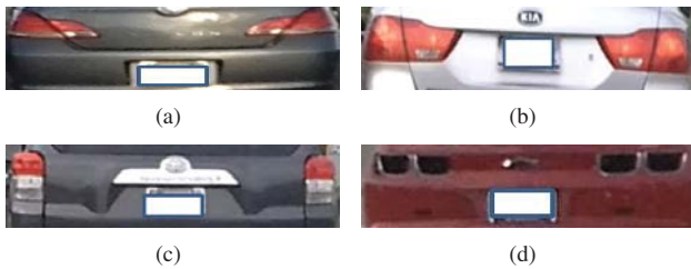
Fig. 5. Examples of tail-light areas used as object-of-interest (manually marked). Notice that the vehicle registration plate is consistently located between the tail-lights either at the same height as or below the tail-light locations.
