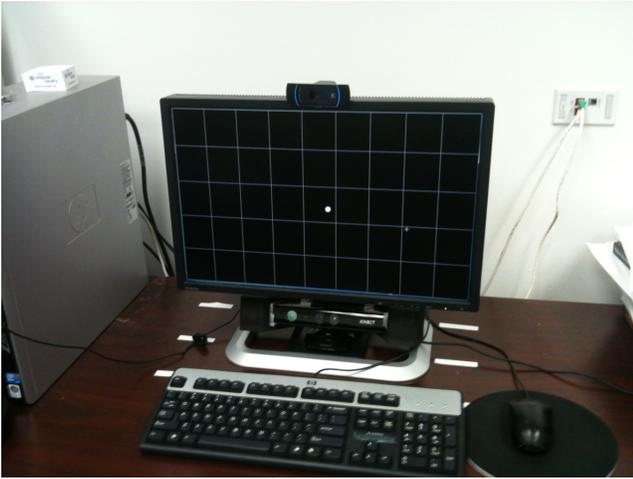
**Figure 1: The data collection includes a 22-inch HP monitor, a Logitech C920 webcam and a Microsoft Kinect for Windows. A green screen is placed behind the subject to provide uniform background.**
