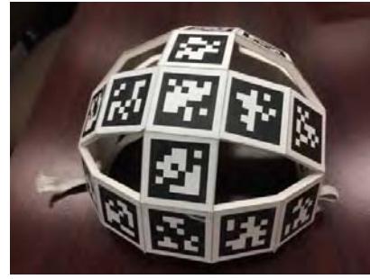
Fig. 6. The Fi-Cap helmet [11], which we use to obtain head pose labels for each frame. A HD camera is placed behind the driver to record the fiducial points in the helmet (Fig. 7(d)).
