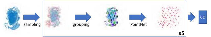
Fig. 15. Diagram of the algorithm proposed by Hu et al. [51] to estimate head pose of the driver using point cloud data. The framework directly uses the point cloud data without projecting the 3D points into 2D spaces.
