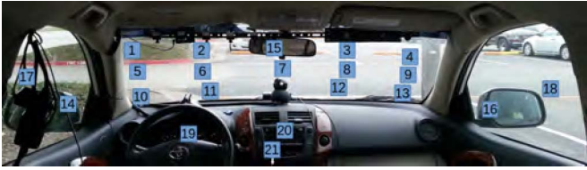
Fig. 3. Location of the target markers placed inside the car. Markers 1-13 are in the windshield. The rest of the markers are in the mirrors (14-16), side of the windows (17-18), speedometer panel (19), radio (20), and gear (21).
