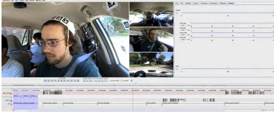
Fig. 10. The corpus uses ELAN as the interface to annotate the recordings. The annotation includes the segments associated with the seven steps in the protocol. It also provides the temporal information for instances when the subject looked at the target markers or objects inside and outside the vehicle.
