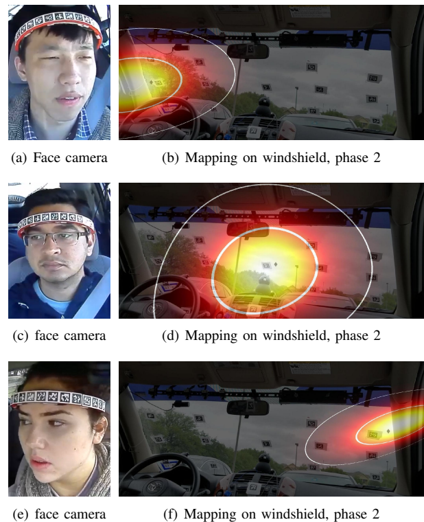
Fig. 6. Example of mapping the gaze region on the windshield (white ellipses give 50% and 95% CIs). The target marker is highlighted with a black circle.
