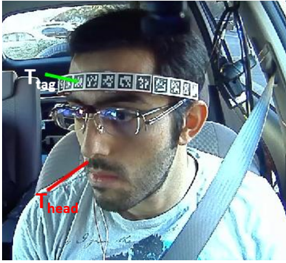
Fig. 4. Transformation from headband orientation to head orientation.
