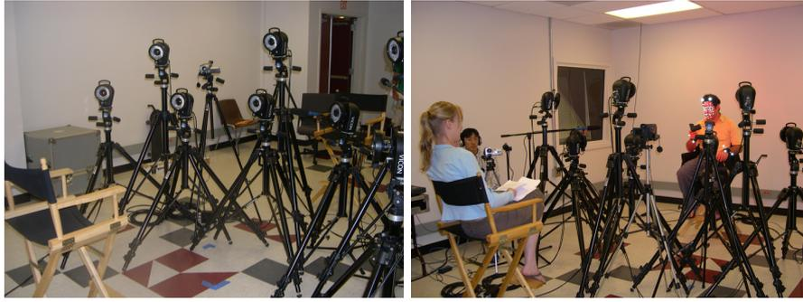
Figure 3. VICON motion capture system with 8 cameras. The subject with the markers sat in the middle of the room, with the cameras directed to him/her. The subject without the markers sat outside the field of view of the VICON cameras, facing the subject with markers.
