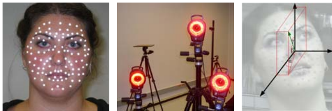
Fig. 1. Audio-visual database collection. The left figure shows the facial marker layout, the middle figure shows the facial motion capture system, and the right figure shows the head motion features extraction.
