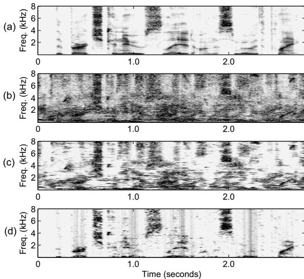
Figure 2: Wideband spectrograms of the clean signal (panel a), corrupted signal (babble, SNR=-5 dB) (panel b), Wiener-processed signal (panel c), and binary masked signal with noise overestimation constraints applied to the enhanced signal (panel d).
