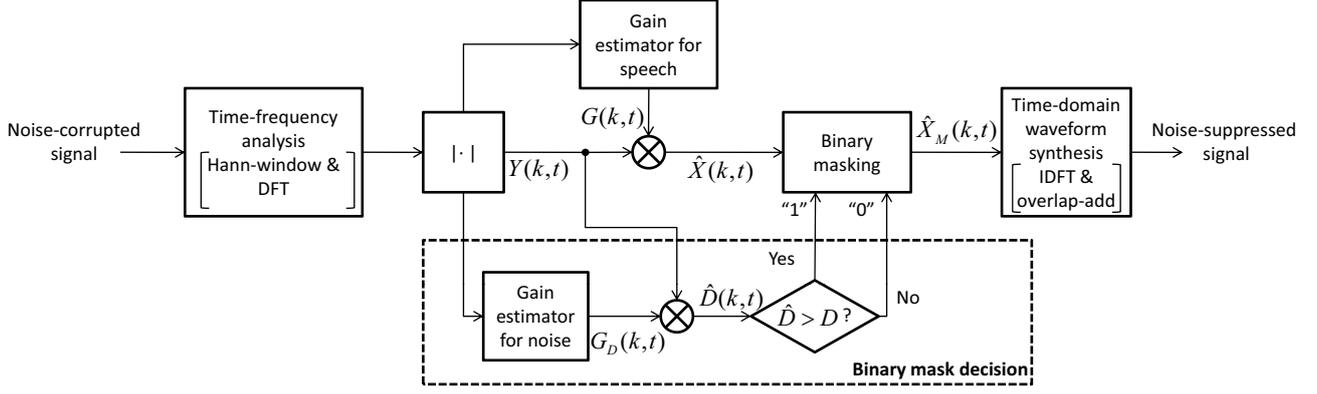
Figure 1: Block diagram of the procedure used for constructing the proposed binary mask based on noise constraints.
