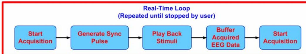
**Figure 9.** Real-time EEG data acquisition implementation.
