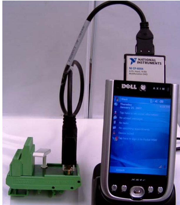
Figure 1. EEG data acquisition setup using the NI CF-6004 compact flash card.
