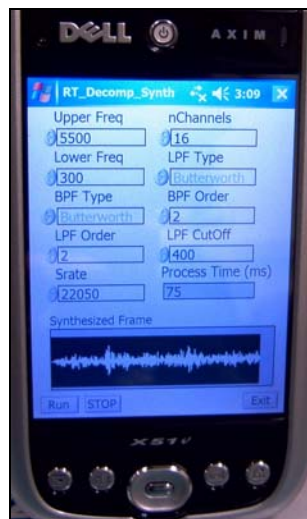
Figure 1. Graphical interface for real-time LabVIEW implementation on the PDA.
