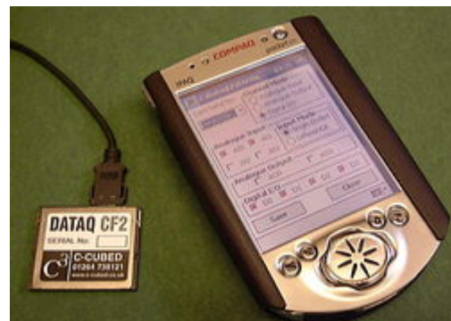
Figure 3. Data acquisition card (Dataq CF2) used for recording EEG on PDA.
