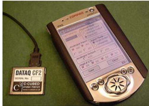
Fig. 2. Data acquisition card (Dataq CF2) used for recording EEG on PDA.
