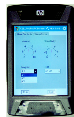
Example user interface designed using LabVIEW
