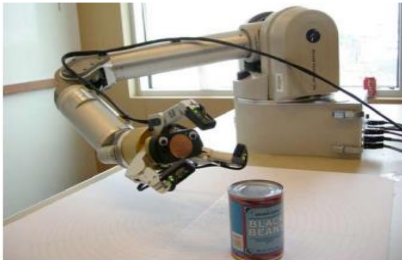
Fig. 1. Photograph of Electric Field Pretouch manipulation system. The system includes a WAM arm and Barrett Hand. Each fingertip contains one of our custom Electric Field Sensing boards and 4 sensing electrodes. Another EF sensing board with one transmit electrode is built into the palm. The palm board also serves as a hub for aggregating sensor data from the fingertips. The palm also contains a camera, which was not used in the experiments reported in this paper. The googly eyes also were not used. A polar coordinate system used for mapping the region of where the grasping procedure succeeds is visible beneath an example object (a can).
