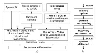
Fig. 2. a) Multimodal system architecture (parts discussed in this work are denoted by bold letters) b) Steps of the proposed microphone array algorithm for speaker tracking and segmentation (proposed algorithm is represented by the mMPF+SOCPD box in multimodal architecture scheme 3a.)
