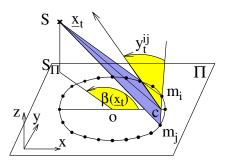
Fig. 3. Microphone array.  $x_t$  - position of source S;  $\prec (m_i cS)$  - true angle between source S and microphone pair  $(m_i, m_j)$ ;  $\beta(x_t)$  - angle that defines source position in the XoY plane;  $y_t^{i,j}$  - Direction of Arrival estimated by microphone pair  $(m_i, m_j)$
