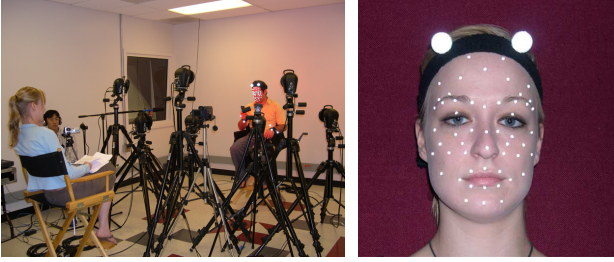
Figure 2: VICON motion capture system with 8 cameras, and an actress showing the markers on the face and headband.
