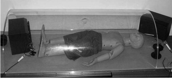
Fig. 6. Test bed used to measure P(z) and S(z) . The targeted application is active noise cancellation of the acoustic noise in MRI machines.
